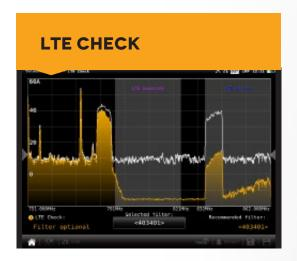
It analyses the impact of the LTE signal on the DTT channels, and detects whether the use of filters is required. Furthermore, it allows spectrum simulation upon the introduction of the LTE filter recommended by the meter itself. A list of filters is displayed for the user to choose the one that best fits his/her requirements.
